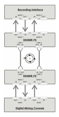
Fig. 3: Redundant network with two DD4MR-FX sending 128 audio channels from console to the recording device and 64 return channels.
